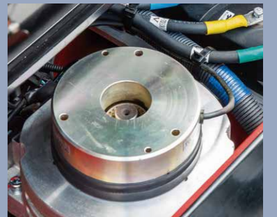
Electrical Park Brake (EPB) system
